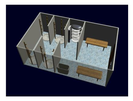
A standard ship's door with a Ge-Y1-E3103 - Intercom System leads into the changing room. A pair of swinging doors leads from the changing room to the showers. A cabinet is located next to the entrance to the shower with clean towels. Another basket in the changing room is for damp towels. The changing room has benches the larger ones have lockers where the crew can store their personal items while showering.
