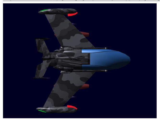
Small egg-like body with rear swept wings that have pods on the end. Wings end past the fuselage. On top of the engine is a retractable boom with connected tail surfaces which add maneuverability and stability in atmosphere.
