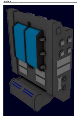
The module has the basic look of a typical backpack; there are a series of four heat sinks located on each side of the backpack and two located on the top. There is a hidden heat sink on the bottom nearest the capacitor.
